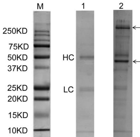
**FIGURE 7.** KYN-modified proteins in mLECs. (A) SDS-PAGE of mLECs lysates. Cell lysate of hemTg mLECs showed high-molecular-weight proteins that were absent in Wt mLECs. (B) SDS-PAGE of immunoprecipitated KYN-modified proteins. Two major KYN-modified proteins (arrows) were detected in hemTg mLECs lysate. Lane M: molecular weight marker; lane 1: Wt mLECs; lane 2: hemTg mLECs. HC, IgG heavy chain; LC, IgG light chain.
